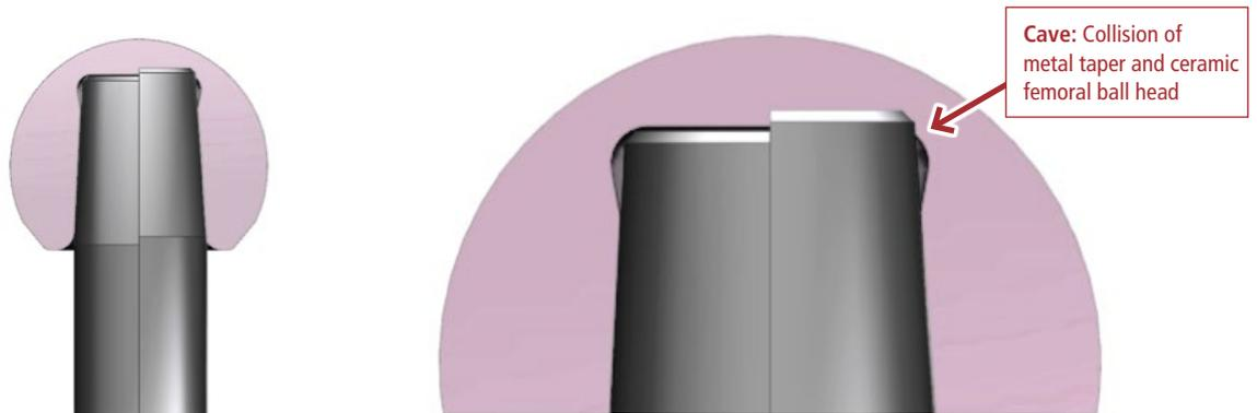
Fig. 4: Compatibility example: Design difference between two nominally similar 12/14 tapers demonstrated with the fit with a ceramic femoral ball head
